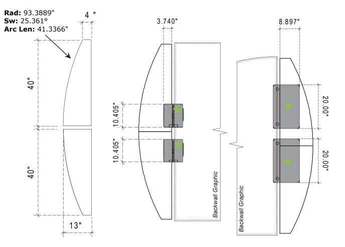
**NOTE:** These dimensions are for graphic layout purposes. Graphic needs to be cut and test fitted to Sacagawea frame. \* Note: The height of Literature Racks can be adjustable.
