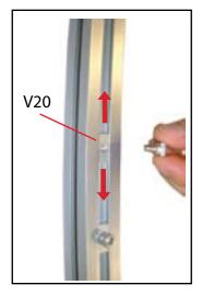
Adjust V20 connector to desired location.
