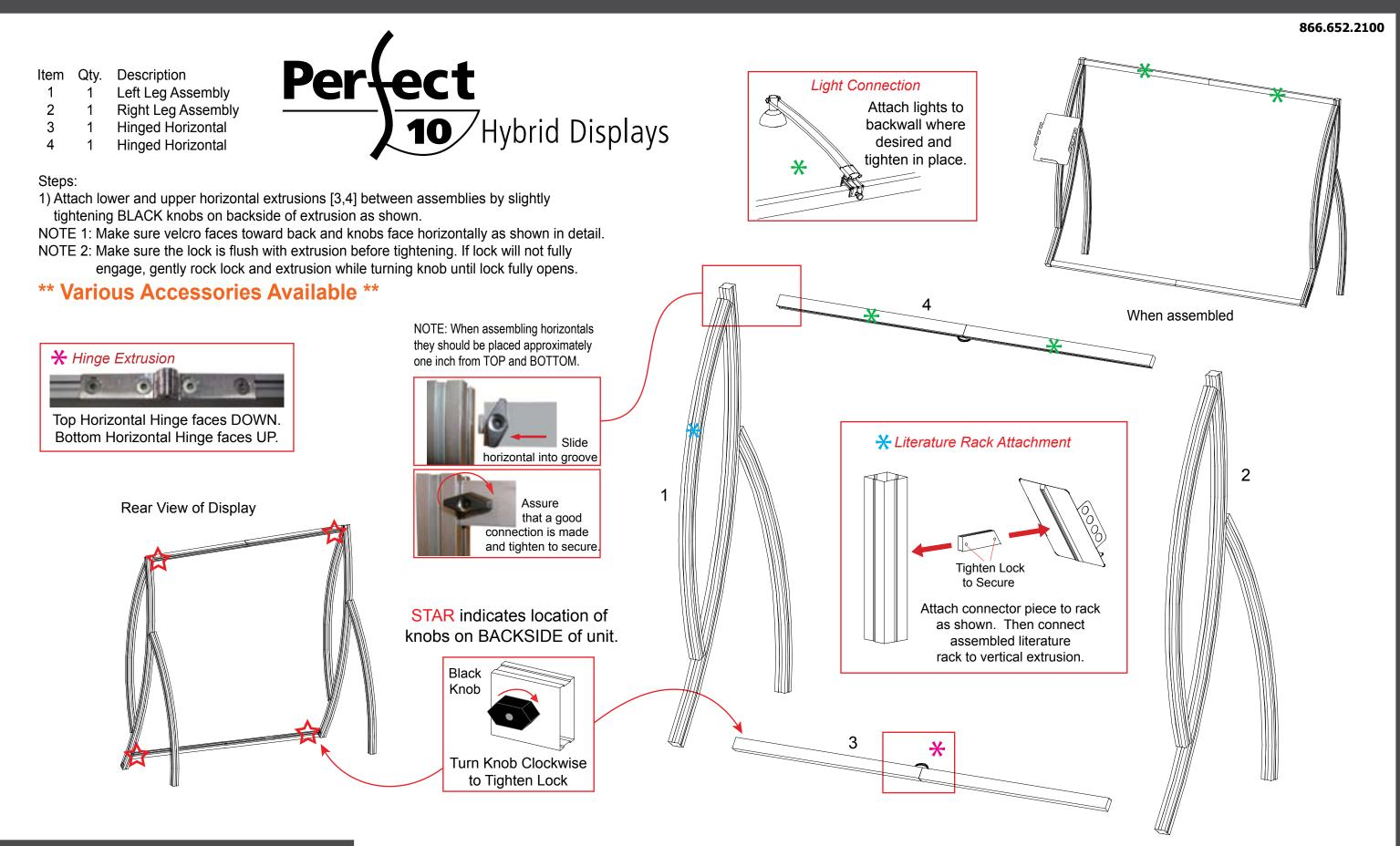
WHEN DISASSEMBLING TIGHTEN ALL KNOBS TO PREVENT LOSS DURING SHIPPING
