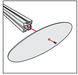
**Base Plate & Extrusion Connection**
