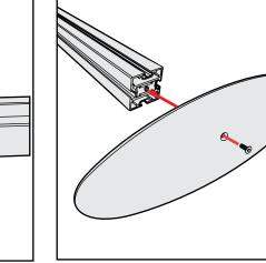
Base Plate & Extrusion Connection
